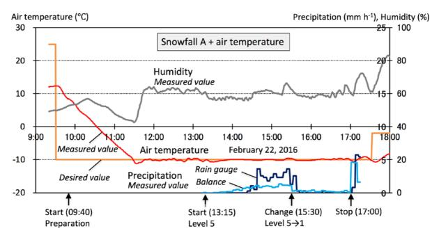
Fig. 11. Time series data for desired and measured precipitation of snowfall A and air temperature, in addition to measured humidity.
