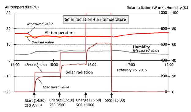
Fig. 14. Time series data for desired and measured solar radiation and air temperature controlled simultaneously.
