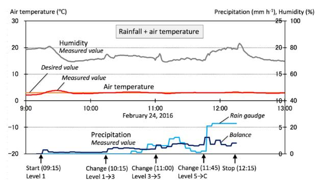
Fig. 13. Time series data for precipitation and air temperature. The numbers indicate the rainfall simulator level used to control the precipitation.
