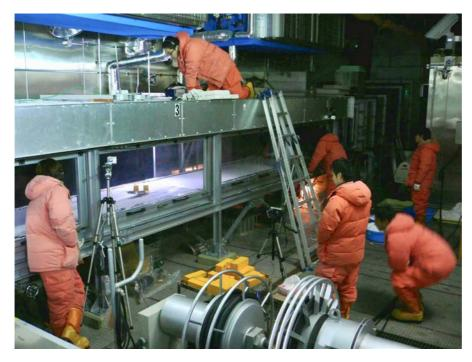
Fig. 7. Wind tunnel with a scale model of the object in the drifting snow layer. The test sections of both sides are comprised of transparent windows and all of the 2-m-wide front windows can be opened.
