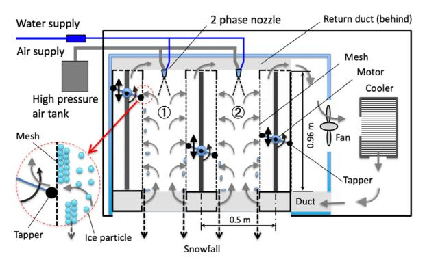
Fig. 3. Schematic of type B snowfall simulator with 2 units. There are 10 units in the simulator installed onto a carrier on the third floor.
