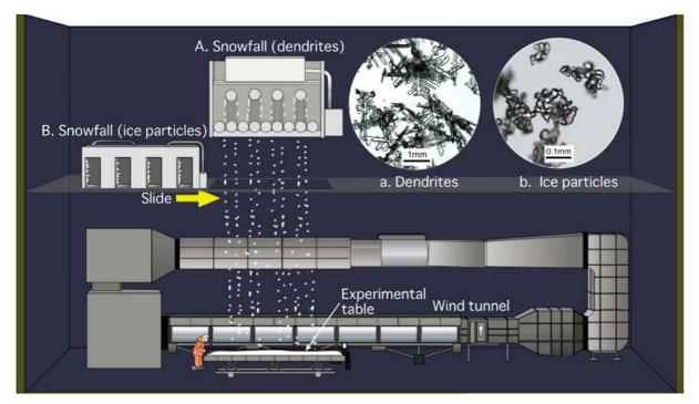
Fig. 1. Two types of snowfall simulators installed on the third floor (original illustration by M. Miura). Type A is fixed, and type B is temporarily at a position just under type A, the latter is used as required. The two circles in the upper right show optical micrographs of the snowfall particles.
