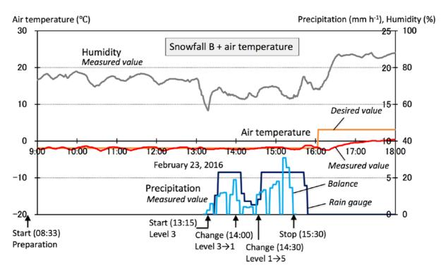
Fig. 12. Time series data for desired and measured precipitation of snowfall B and air temperature, in addition to measured humidity.
