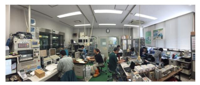
Fig. 10. CES Control room. An operator (left) monitors the control panel and a technician (left back) supports data collection for the collaborators who typically provide their original instruments (right). The cold room can be seen through the window on the left.
