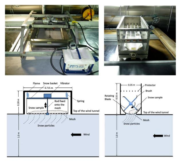
Fig. 8. Small snowfall machines used to sieve snow particles into the wind tunnel from the top window. Left: vibrational type, Right: rotating-brush type. Bottom figures show the snowfall machine schematics.
