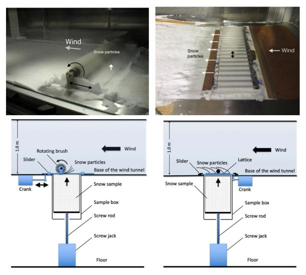
Fig. 9. Snow seeders in the wind tunnel. Left: rotating-brush type, Right: reciprocating type. Bottom figures show the snow seeder schematics. Dimensions of the sample box for both types are 0.2 m in length  $\times$  0.77 m in width  $\times$  0.3 m in depth.
