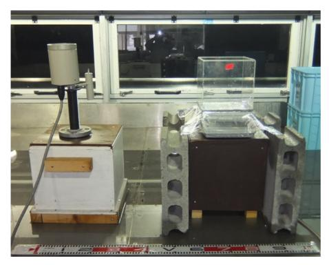
Fig. 5. Rain gauge (left) and balance with a square vessel (right).
