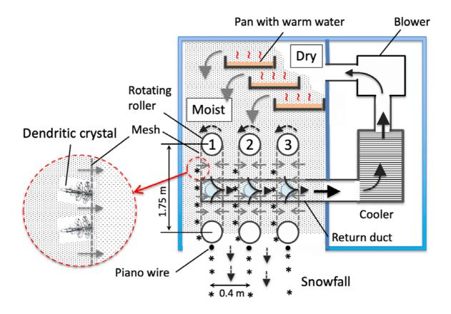
Fig. 2. Schematic of type A snowfall simulator with 3 units. There are 12 units in the simulator installed on the third floor.
