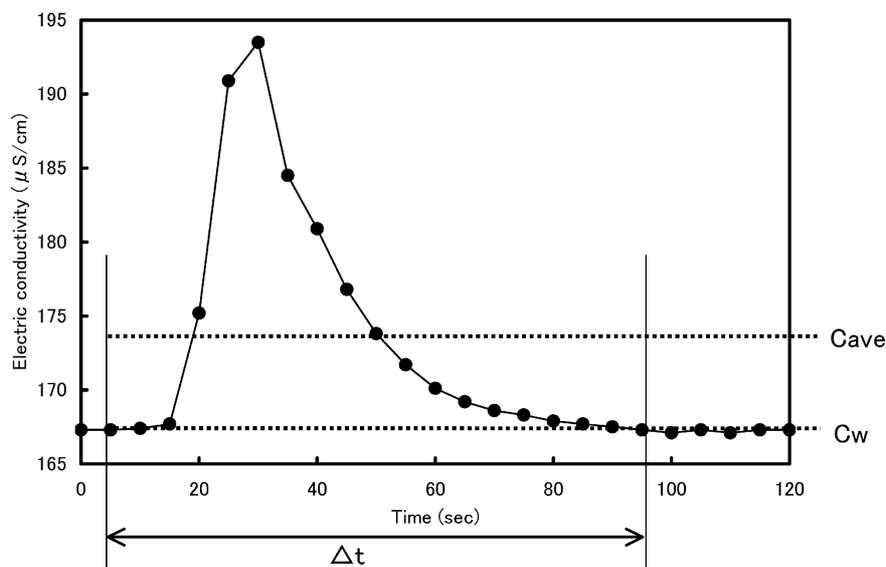
Fig. 3. Example of fluctuation of electric conductivity, when the discharge was measured by salt water dilution gauging method.  $t$ ,  $C_w$ , and  $C_{ave}$  correspond with parameters in Eq. (1).
