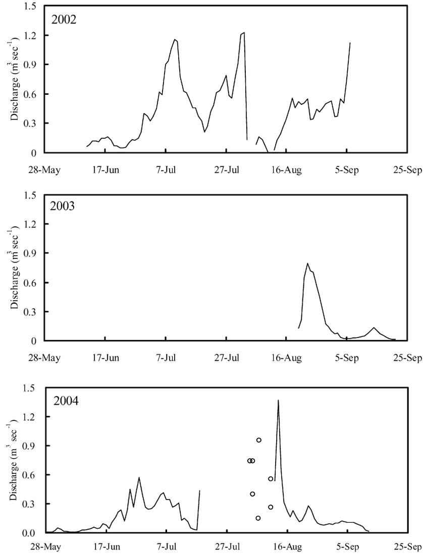
Fig. 5. Variation of discharge during melting season in 2002, 2003 and 2004. White circle shows instantaneous value (not daily) of observed discharge calculated manually from observed water level.
