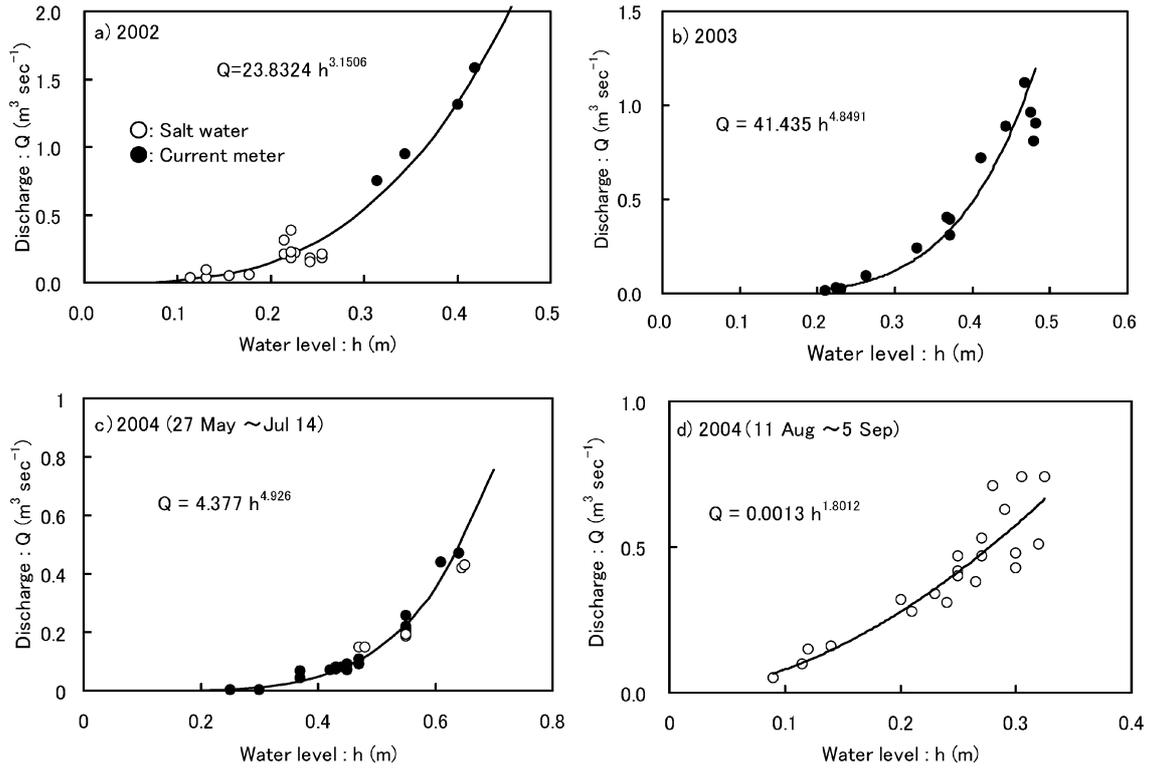
Fig. 4. Relationships between water level and discharge observed from 2002 to 2004. Discharge measurement by salt water dilution gauging method is shown by empty circles and velocity-area method using the water current meter by solid circles.
