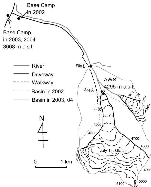
Fig. 2. Observed basin in 2002 and 2003–2004. Sites A and B indicate discharge measurement sites in 2002 and in 2003, 2004, respectively. Empty circles show location of Automatic Weather Station. Lysimeters were set up at AWS site and Base camp in 2004.
