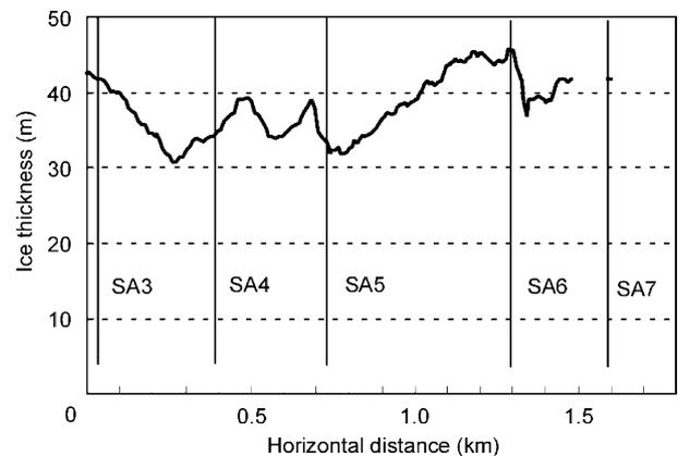
Fig. 6. Ice thickness profile along the study sites showing in Fig. 3. The thickness was calculated based on a radio propagation speed of 169 m  $\mu$  sec<sup>-1</sup>.
